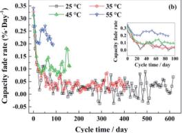
Fig. 10 (a) The capacity retentions of the LiFePO<sub>4</sub>/graphite full cells at different temperatures with continuous cycling days, (b) the capacity fade rate at each test temperature during cycling. 113
