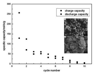
Fig. 16 Cyclic performance of  $\rm Li_2MnSiO_4$  synthesized by solid state method tested at C/16 rate to a cut-off voltage between 1.5 and 4.8 V.<sup>152</sup> The inset shows FESEM micrographs of (a)  $\rm Li_2MnSiO_4$  and (b)  $\rm Li_2MnSiO_4/C$ .
