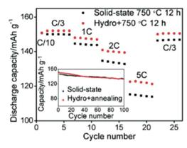
Fig. 19 Comparison of two materials, one was sintered for 12 h at 750  $^{\circ}$ C and the other was prepared by hydrothermal method then sintered for 12 h at 750  $^{\circ}$ C.<sup>159</sup>
