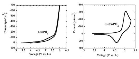
Fig. 14 Cyclic voltammetry of LiNiPO<sub>4</sub> and LiCoPO<sub>4</sub> at a scan rate of 0.2 mV s $^{-1.135}$
