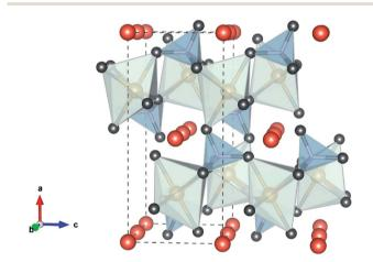
Fig. 9 Polyhedral representation of the olivine structure. FeO<sub>6</sub> (light green), PO<sub>4</sub> (gray), and the Li<sup>+</sup> (orange) "by VESTA".
