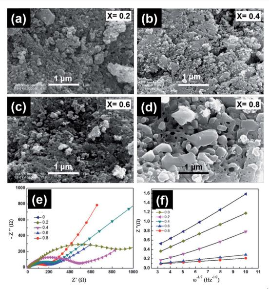
Fig. 13 (a-d) FESEM images, (e) impedance spectra, and (f) the relationship between Z'' and the square root of frequency ( $\omega^{-1/2}$ ) in the lowfrequency region for LiMn<sub>1-x</sub>Fe<sub>x</sub>PO<sub>4</sub> at different compositions.<sup>131</sup>
