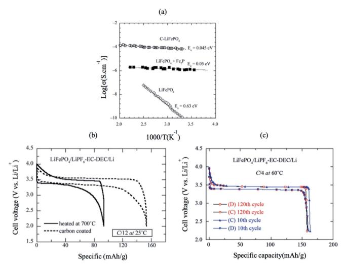
Fig. 12 (a) Electronic conductivity of pure LiFePO<sub>4</sub>, Fe<sub>2</sub>P-containing sample and C/LiFePO<sub>4</sub>. (b) The electrochemical profiles at C/12 of non-coated and heated at 700 °C LiFePO<sub>4</sub>//Li cells (c) electrochemical performance of the C-LiFePO<sub>4</sub>//Li cell operating at 60 °C. Charge-discharge cycling was conducted at the C/4 rate (about 35 mA g<sup>-1</sup>) in the voltage range 2.2–4.0 V vs. Li<sup>0</sup>/Li<sup>+</sup>.<sup>123</sup>
