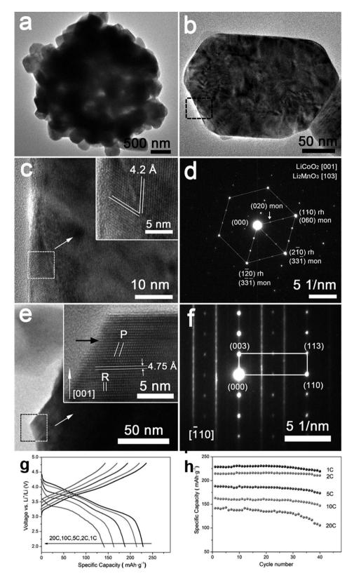
Fig. 8 (a–f) Hierarchical  $Li_{1.2}Ni_{0.2}Mn_{0.6}O_2$  nanoplates with exposed {010} planes as high-performance cathode material for lithium-ion batteries, (g) discharge curves of half cells based on the  $Li_{1.2}Ni_{0.2}Mn_{0.6}O_2$  hierarchical structure nanoplates at 1C, 2C, 5C, 10C, and 20C rates after charging at C/10 rate to 4.8 V, and (h) the rate capability at 1C, 2C, 5C, 10C, and 20C rates.<sup>88</sup>
