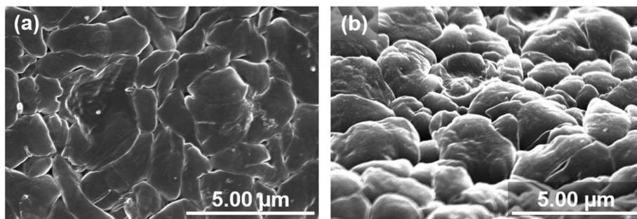
Fig. 4 SEM image of the deposited lithium surface pressed with 3.14 MPa for 2 days. Lithium was electrodeposited on a copper substrate at a current density of  $1.0 \text{ cm}^{-2}$  for 1 hour. These were observed from (a) vertical and (b) oblique angles, respectively.
