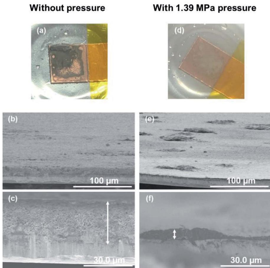
Fig. 8 Surface optical and cross-sectional SEM images of the copper electrode after the 1<sup>st</sup> plating/stripping cycle at  $1.0 \text{ mA cm}^{-2}$  for 1 h without pressure (a–c), and under a pressure of 1.39 MPa (d–f).
