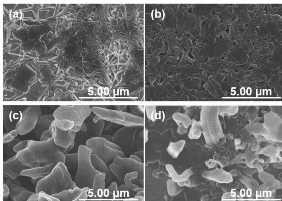
Fig. 6 SEM images of the electrodeposited lithium when the pressure applied to the cell during lithium plating reaction. (a and b) Morphologies of electrodeposits plated at  $1.0 \text{ mA cm}^{-2}$  for 30 minutes under 1.39 MPa after lithium plating at  $1.0 \text{ mA cm}^{-2}$  for 30 minutes without pressure. (c and d) Those plated at  $1.0 \text{ mA cm}^{-2}$  for 30 minutes without pressure after lithium plating at  $1.0 \text{ mA cm}^{-2}$  for 30 minutes under 1.39 MPa.
