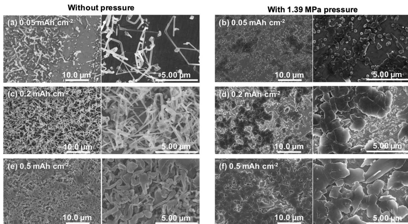
Fig. 5 SEM images of copper electrode after lithium plating with and without uniaxial pressure. Electrodeposition at (a and b)  $0.05 \text{ mA h cm}^{-2}$ , (c and d)  $0.2 \text{ mA h cm}^{-2}$  and (e and f)  $0.5 \text{ mA h cm}^{-2}$  was performed at a current density of  $1.0 \text{ mA cm}^{-2}$ .
