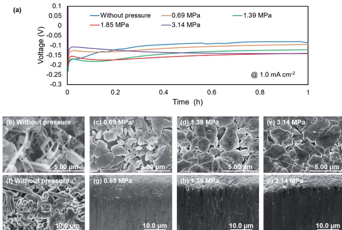
Fig. 2 Characterization of lithium metal plating behavior on a copper substrate at 1.0 mA cm<sup>-2</sup> under various uniaxial pressures. (a) First discharge curves for the plating reaction under various pressures. SEM images of electrodeposited lithium without pressure (b and f), and under pressures of 0.69 MPa (c and g), 1.39 MPa (d and h), and 3.14 MPa (e and i). Upper (b–e) and lower (f–i) panels are surface and cross-section images.
