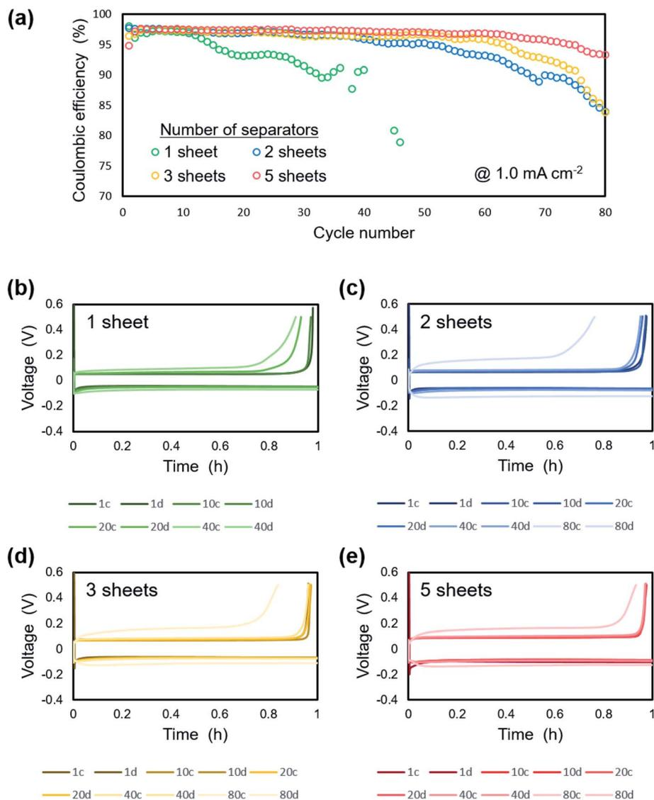
Fig. 11 Electrochemical performance of lithium plating/stripping on copper substrate at  $1.0 \text{ mA cm}^{-2}$  under a pressure of  $1.39 \text{ MPa}$ . (a) Cycle dependence of coulombic efficiency with various numbers of separator sheets. Charge/discharge curves of Li/Cu cells with (b) 1, (c) 2, (d) 3 and, (e) 5 separator sheets.
