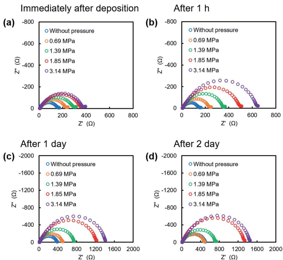
Fig. 3 Nyquist plots of the Li/Cu pouch cell after the lithium plating reaction on the copper electrode at  $1.0 \text{ mA h cm}^{-2}$ . EIS measurements were conducted (a) immediately, and after various storage times of (b) 1 h, (c) 1 day, and (d) 2 days.
