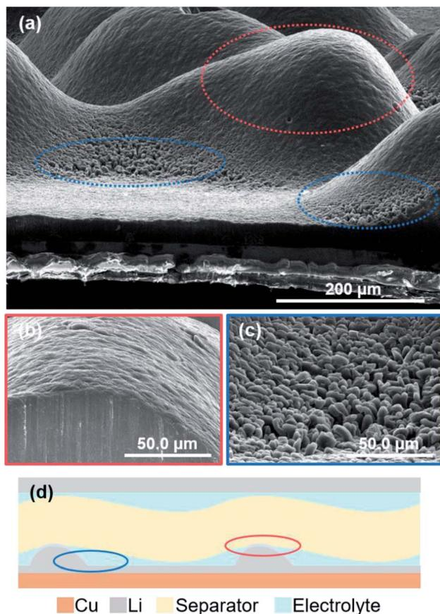
Fig. 9 (a) Cross-sectional SEM images of the electrodeposited lithium metal after plating on the copper substrate at  $15 \text{ mA h cm}^{-2}$  under a pressure of  $1.39 \text{ MPa}$ . Expanded images at (b) the convex portion and (c) the concave portion. (d) Schematic diagram of the morphology of electrodeposited lithium in contact with a separator with poor flatness.
