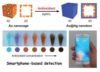
Fig. 3 The sensing principle of antioxidant based on the morphological change of An nanocage upon the reduction of  $AgNO_3$  producing Au@Ag nanobox in presence of antioxidants. Adapted from ref. 48 with permission from Royal Society of Chemistry, Copyright 2018
