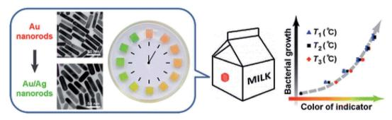
Fig. 13 Time—temperature indicator based on silver growth on gold nanorods creating a change in color related to microbial growth which is governed by time and temperature. The clock illustration shows Ag/Au nanorods-hydrogel cubes arranged in a Petri dish indicating the color change over time. Reprinted with permission from ref. 135. Copyright (2013) American Chemical Society.
