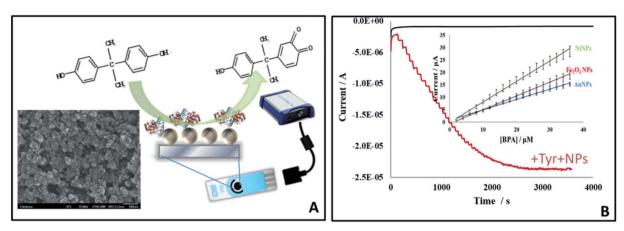
Fig. 5 Enzyme-based detection of BPA by NP amplification using screen printed electrodes modified with Au, Ni or  $Fe_2O_3$  NPs: sensor design (A) and amperometric response with comparative calibration curve (B) showing differential responses to the three types of NPs of which Ni NPs showed the highest sensitivity (schematic summarizing detection platform and results reported in ref. 33).
