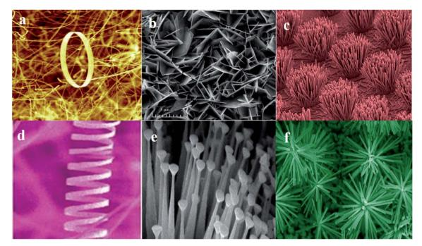
Fig. 1 Representative structures of some nano-materials: (a) nanorings, <sup>228</sup> (b) nanopellets, <sup>229</sup> (c) nanorods, <sup>230</sup> (d) nanosprings, <sup>228</sup> (e) nanonails, <sup>231</sup> (f) nanoflower. <sup>232</sup>
