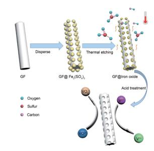
Fig. 1 Schematic of the preparation process of GF@P electrode
