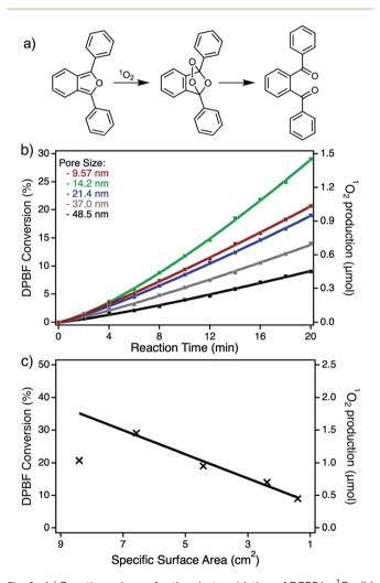
Fig. 6 (a) Reaction scheme for the photooxidation of DPBF by  $^{1}O_{2}$ . (b) Photocatalytic DPBF oxidation over time by npAu photocatalytic coatings with pore sizes of 9.57 nm (red), 14.2 nm (green), 21.4 nm (blue), 37.0 nm (grey) and 48.5 nm (black). (c) Plot of the maximum conversion after 20 min vs. the specific surface area of the corresponding hybrid for visualization of diffusion limitation and mass transport phenomena.
