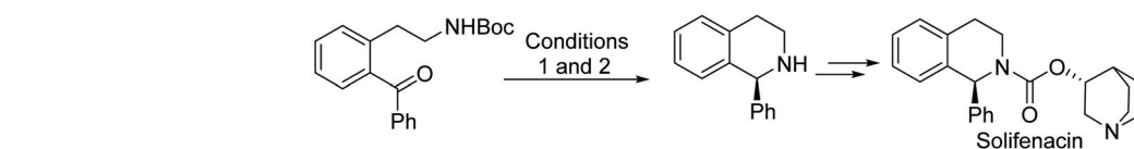
Fig. 3 Reductions of 1-aryl-3,4-dihydroisoquinolines and enantioselective synthesis of Solifenacin.
