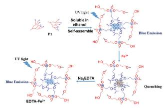
Fig. 7 The mechanism of P1 as a Fe<sup>3+</sup> probe: "turn off" (fluorescence quenching after the formation of the P1-Fe3+ complex); "turn on" (fluorescence restored after the formation of the EDTA-Fe<sup>3+</sup> complex and the breaking of the P1-Fe3+ complex).
