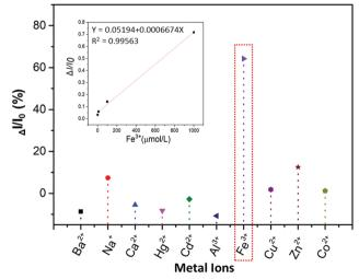
Fig. 6 Luminescence quenching rate ( $\Delta I/I_0$ ) of the 15 mg mL<sup>-1</sup> P1 water– ethanol solution with different metal ions (1  $\times$  10<sup>-3</sup> mol L<sup>-1</sup>), and the relationship between  $\Delta I/I_0$  and the concentration of Fe<sup>3+</sup>.
