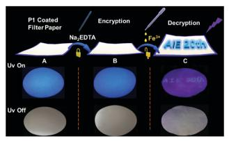
Fig. 8 Photographs of (A) P1 coated security paper; (B) security paper after writing with  $Na_2EDTA$ ; (C) security paper treated with  $FeCl_3$  (1  $\times$  $10^{-3}$  mol L<sup>-1</sup> water-ethanol solution) under natural light or under the irradiation of 365 nm UV light.
