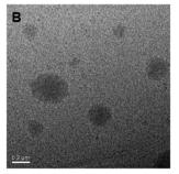
Fig. 5 TEM micrographs of self-assembled morphology of P1 in ethanol with the concentration at (A) 5 mg  $mL^{-1}$  and (B) 50 mg  $mL^{-1}$ .
