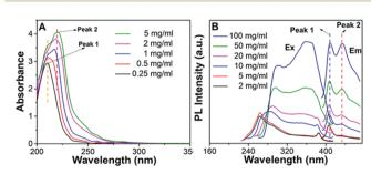
Fig. 2 (A) UV-vis absorption spectra of P1 ethanol solution with the concentration increased from 0.25 mg mL<sup>-1</sup> to 5 mg mL<sup>-1</sup>; (B) excitation ( $\lambda_{em}$  = 406 nm) and emission ( $\lambda_{ex}$  = 360 nm) spectra of **P1** ethanol solution with the concentration increased from 2 mg mL<sup>-1</sup> to 100 mg mL<sup>-1</sup>.
