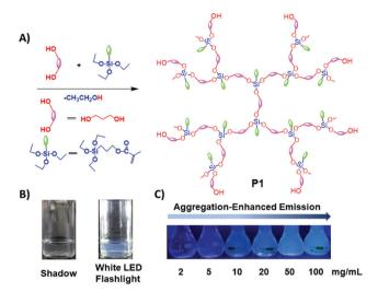
Fig. 1 (A) Synthetic route toward P1; (B) 15 mg mL<sup>-1</sup> P1 ethanol solution under white LED flashlight or shadow; (C) P1 ethanol solution with different concentrations under 365 nm UV light.
