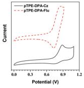
Fig. 3 Cyclic voltammograms of pTPE-DPA-Cz and pTPE-DPA-Flu measured in DCM containing 0.1 M tetra-n-butylammonium hexafluorophosphate. Scan rate: 100 mV s<sup>-1</sup>.
