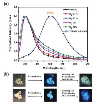
Fig. 8 (a) Normalized PL spectra of TPDBM doped PMMA film in N<sub>2</sub>/O<sub>2</sub> mixed gas with different volume ratios. (b) Images of TPDBM solid powder under different treatment conditions.
