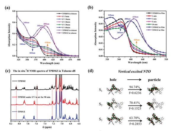
Fig. 6 In situ UV spectra of TPDBM (a) in toluene solution and (b) as a film. (c) In situ <sup>1</sup>H NMR spectra of TPBMZ. (d) The natural transition orbital (NTO) distributions of **TPBMZ** relating to  $S_0 \rightarrow S_1$ ,  $S_0 \rightarrow S_2$  and  $S_0 \rightarrow S_3$  excitations at the TD-oB97X/6-31G(d,p) level using  $S_0$  state geometry.
