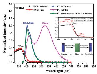
Fig. 2 UV-vis and PL spectra of TPDBM in toluene solution and film states; the inset shows the excitation spectra of TPDBM film at 430 nm and 520 nm.
