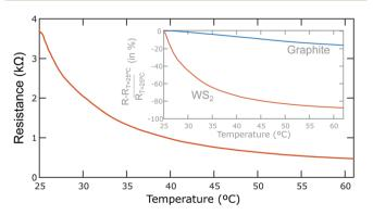
Fig. 4 Temperature dependence of the resistance of WS<sub>2</sub>-on-paper thermoresistive devices. (a) Resistance vs. temperature for a WS<sub>2</sub>-on-paper device with pencil-drawn interdigitated devices. (inset) Comparison between the resistance vs. temperature curves measured for the WS<sub>2</sub> and a graphite thermoresistive devices on paper.
