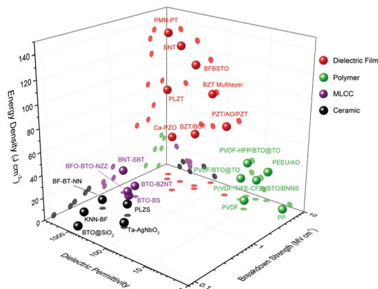
**Fig. 2** Comparison of dielectric permittivity, breakdown and energy storage performance between representative dielectric films, polymers (and polymer-based composites), MLCC, and ceramics.<sup>17–25,27–38</sup>
