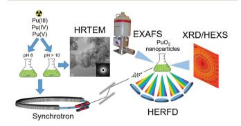
Fig. 1 The schematic illustration of the research methodology applied to PuO2 NPs studies. PuO2 NPs synthesized from different precursors (Pu(III), Pu(IV) and Pu(V)) and at pH 8 and pH > 10 were analysed with HRTEM and various synchrotron techniques (EXAFS, XRD, HEXS and HERFD)
