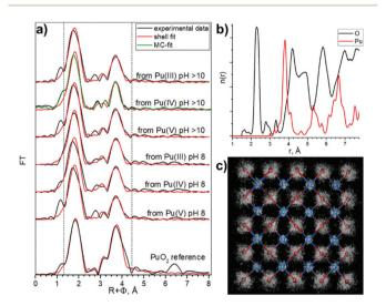
Fig. 4 Pu L<sub>3</sub> EXAFS results. (a) Pu L<sub>3</sub> EXAFS spectra  $\chi(R)$  fit results, Fourier transform (FT) magnitude of experimental EXAFS data (black) and a one Pu-O, one Pu-Pu shell fit (red), Monte-Carlo simulations fit (green). The area of the shell fit in R-space is marked with two dashed lines, (b) MC simulation output: radial particle distribution function (n(r))for Pu-O and Pu-Pu, (c) 3D structural refinement based on bulk PuO2 structure
