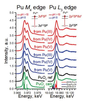
Fig. 3 Pu  $M_4$  and  $L_3$  HERFD experimental data. Data recorded for six  $PuO_2$  NPs samples and compared with a  $PuO_2$  reference and theoretical calculations, using AIM approximation (left) and FEFF code (right). The density of states is plotted at the bottom for clarity.
