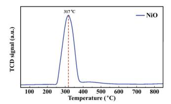
Fig. 2  $H_2$  TPR profile of the NiO/ $\gamma$ -Al<sub>2</sub>O<sub>3</sub> catalyst.
