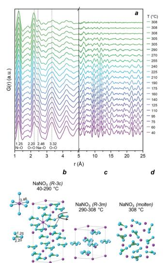
Fig. 2 (a) PDF of NaNO $_3$  heated from 40 °C to 308 °C in N $_2$  and hold at 308 °C for 10 min; (b) illustration of the NaNO $_3$   $R\bar{3}c$  (ICSD: 180912) crystalline structure and short-range correlations below 2.5 Å; (c)  $R\bar{3}m$  (ICSD: 180920) crystalline structure; (d) schematic representation of the molten NaNO $_3$  state. Color legend: blue – oxygen, purple – sodium, green – nitrogen.
