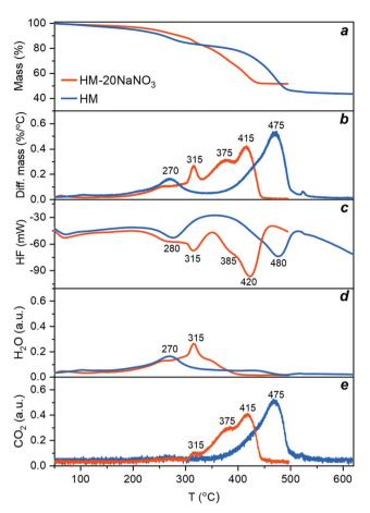
Fig. 1 Thermal decomposition of HM (blue) and HM-20NaNO $_3$  (red) during thermal treatment in N $_2$  (10 °C min $^{-1}$ ): (a) mass loss and (b) rate of mass loss determined by TGA; (c) heat flow and simultaneous measurement of (d) H $_2$ O and (e) CO $_2$  released during the reaction.
