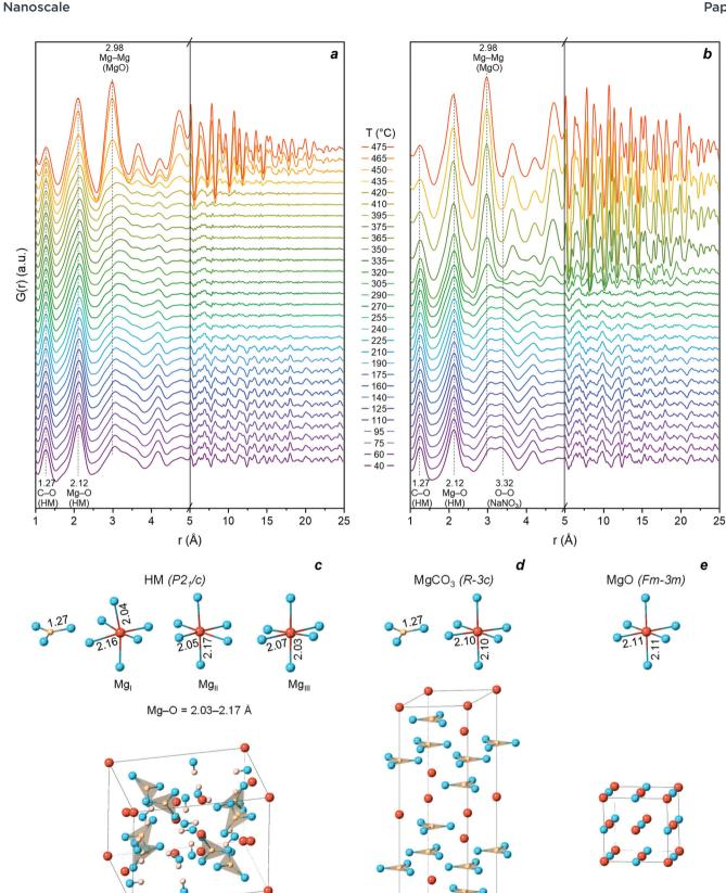
Fig. 3 PDF obtained while heating (a) HM and (b) HM-20NaNO<sub>3</sub> from 40 °C to 475 °C in N<sub>2</sub>. Illustration of the crystal structure and short-range correlations below 2.5 Å of (c) HM (P2<sub>1</sub>/c, ICSD: 920); (d) crystalline-MgCO<sub>3</sub> (R3c, ICSD: 40117); (e) MgO (Fm3m, ICSD: 9863). Color legend: blue – oxygen, red - magnesium, pink - hydrogen, yellow - carbon.
