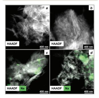
Fig. 5 HAADF-STEM images along with Na EDX maps of (a) as-received HM, (b) HM after thermal treatment in N2 at 450 °C, (c) as-prepared  $HM-20NaNO_3$  and (d)  $HM-20NaNO_3$  after thermal treatment in  $N_2$  at 450 °C.
