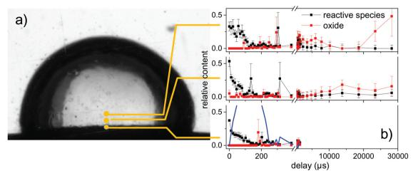
Fig. 6 (a) Videography still of the vapour bubble at a delay of  $114 \mu s$ . The dots indicate the positions, where the TR-XAFS spectra were acquired. (b) Time-resolved contributions of the reactive species and ZnO to the XANES part of the spectra as derived by a least squares fit.
