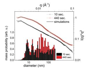
Fig. 2 Selected SAXS measurements (symbols) after given time of batch processing of 10 and 440 seconds. The fit results from the particle size distribution are shown as lines. Lower left: Histogram of the massweighted particle size distribution as determined by the fits.
