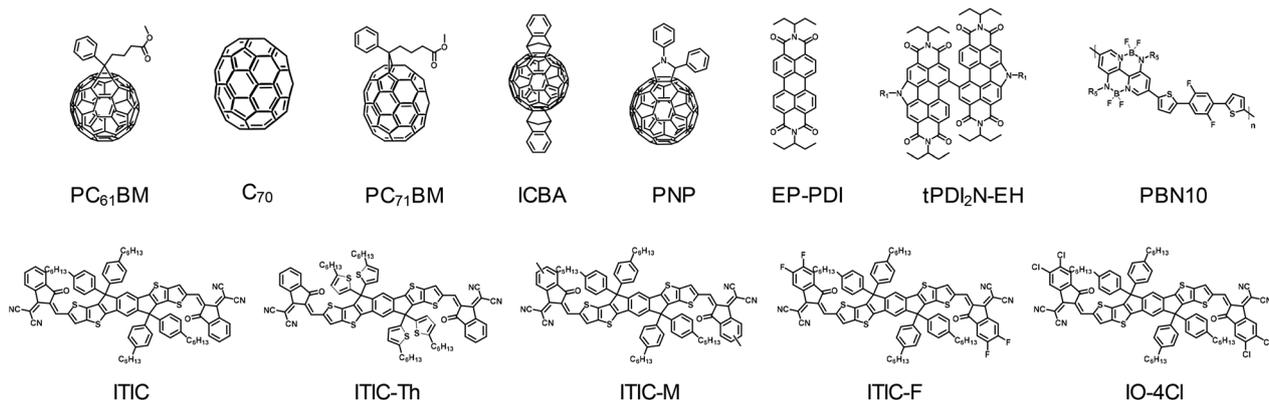
**Fig. 4** Acceptor structures for indoor organic photovoltaic devices.
