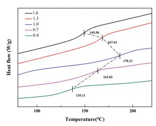
Fig. 4 DSC curves of different molar ratios of the A/E in the blend.
