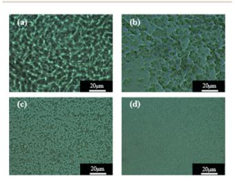
Fig. 1 OM images of the blend system at 85  $^{\circ}$ C for different curing times: (a) 38 min, (b) 51 min, (c) 64 min, and (d) 89 min.
