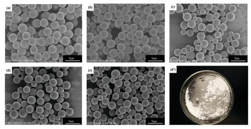
Fig. 2 SEM images of Ems with different molar ratios of the A/E in the blend and photograph of Ems (A/E = 1.3): (a) 0.4; (b) 0.7; (c) 1.0; (d and d') 1.3; and (e) 1.6.
