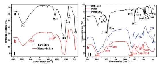
Fig. 4 (I) FT-IR spectrum of bare and silanized silica, (II) FT-IR spectra of (a) DMHAAB, (b) PASD and (c) PASD-SiO<sub>2</sub>.
