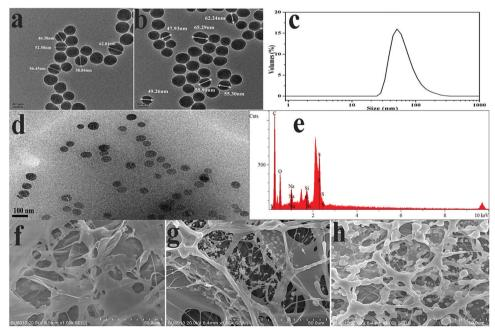
Fig. 6 TEM micrographs of (a) pure SiO2 and (b) modified SiO2, (c) particle size distribution of modified SiO2, (d) TEM image of PASD-2%SiO2, (e) elemental analysis of PASD-3%SiO2, SEM images of (f) 0.5 wt% PASD, (g) 0.5 wt% PASD-2%SiO2 and (h) 0.5 wt% PASD-3%SiO2.
