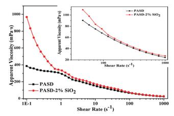
Fig. 12 Effect of the shear rate on apparent viscosity of PASD and PASD-2%SiO<sub>2</sub>. Inset showed the apparent viscosity at a high shear rate.
