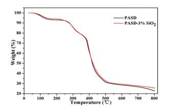
Fig. 8 Thermal gravimetric curves of PASD and PASD-3%SiO<sub>2</sub>.
