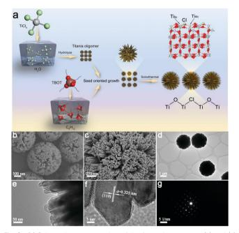
Fig. 2 (a) Schematic representation of the formation process, (b) and (c) SEM, (d) and (e) TEM, (f) HRTEM images, and (g) the selected-area electron diffraction (SAED) pattern of the single-crystal rutile TiO2 nanorodassembled radial microspheres with chemisorbed Cl on the surface.
