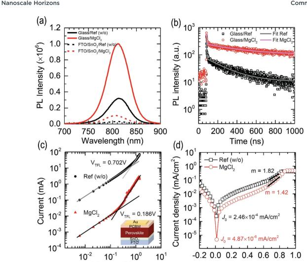
Fig. 7 (a) Steady-state photoluminescence (PL) of the FAPbI<sub>3</sub> film with and without MgCl<sub>2</sub> deposited on a glass substrate and SnO<sub>2</sub>-coated FTO substrate. (b) Time-resolved PL (TRPL) for the FAPbI<sub>3</sub> film with and without MgCl<sub>2</sub> on a glass substrate. Dark current density (J)-voltage (V) curves for (c) the FTO/SnO<sub>2</sub>/FAPbI<sub>3</sub> (with or without MgCl<sub>2</sub>)/PCBM/Au electron-only device and (d) the full solar cell device.
