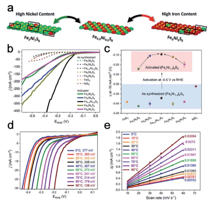
Fig. 6 (a) Schematic surface area of  $(Fe_xNi_{1-x})_9S_8$  with different Ni/Fe ratios. (b) LSV curves and (c)  $\eta$  for synthesized and activated  $(Fe_xNi_{1-x})_9S_8$  samples. (d) LSV curves of  $Fe_{4.5}Ni_{4.5}S_8$  at different temperatures. (e) Charging current density differences  $(\Delta J = j_a - j_c)$  plotted. Reproduced with permission. Copyright 2018, American Chemical Society.
