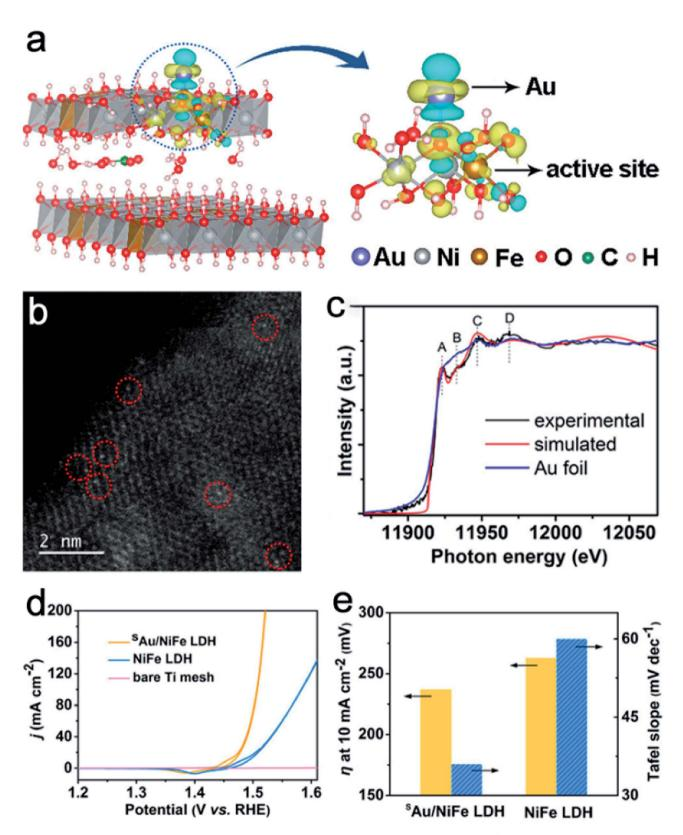
Fig. 3 (a) Differential charge densities of Ni-Fe LDH with and without Au atoms. (b) HAADF-STEM of SAu/Ni-Fe LDH. (c) Au L3-edge XANES spectra of  $^{s}$ Au/Ni-Fe LDH and Au foil. (d) Polarization curves of  $^{s}$ Au/Ni-Fe LDH, pure Ni-Fe LDH and Ti mesh. (e)  $\eta$  at 10 mA cm<sup>-2</sup> and Tafel slope for <sup>5</sup>Au/Ni-Fe LDH and Ni-Fe LDH. Reproduced with permission. <sup>50</sup> Copyright 2018, American Chemical Society.
