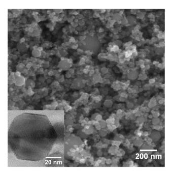
Fig. 1 SEM image of the initial  $\gamma$ -Fe<sub>2</sub>O<sub>3</sub> nanoparticles. The inset shows TEM image of a single nanoparticle.
