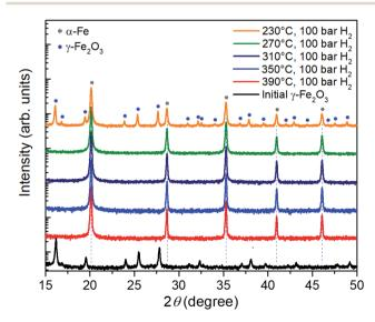
Fig. 2 XRD patterns of the  $\gamma$ -Fe<sub>2</sub>O<sub>3</sub> nanoparticle powder before and after three-hour reduction in hydrogen at a pressure of 100 bar and temperatures between 230 °C and 390 °C.
