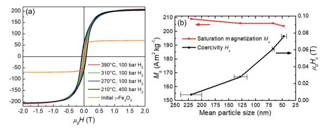
Fig. 8 (a) Hysteresis loops for the initial  $\gamma$ -Fe<sub>2</sub>O<sub>3</sub> and  $\alpha$ -Fe particles produced by hydrogen reduction at 390 °C, 310 °C, 270 °C and 210 °C. (b) Saturation magnetization  $M_s$  and coercivity  $H_c$  at room temperature as a function of the particle size for the hydrogen reduced  $\alpha$ -Fe nanoparticles.
