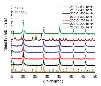
Fig. 3 XRD patterns of the  $\gamma$ -Fe<sub>2</sub>O<sub>3</sub> nanoparticle powders after three-hour reduction at temperatures of 210°C–230 °C and hydrogen pressures in the range between 100 bar and 530 bar.
