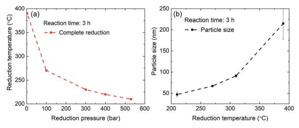
Fig. 5 Summary of the results from hydrogen reduction experiments. (a) Gradual increase in hydrogen pressure enables lowering of the reaction temperature. (b) At lower reduction temperatures particle growth is minimized.
