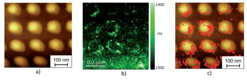
Fig. 6 (a) AFM topology image of the Au nanodisk array with CdSe NCs. (b) TERS intensity image of LO phonon mode from CdSe NCs, obtained simultaneously with the AFM image shown in (a). (c) Superposition of the AFM image and TERS intensity from the same sample area indicating that the strong TERS signal originates predominantly from the Au nanodisk edges. (c) is created by overlaying the background subtracted TERS map (b) on top of the AFM topography (a).
