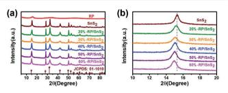
Fig. 1 XRD patterns of (a) full spectra and (b) magnified spectra of samples RP,  $SnS_2$ , and x-RP/ $SnS_2$ .
