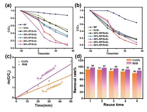
Fig. 2 Comparison of the effect of photocatalytic simultaneous removal of (a)  $Cr(v_1)$  and (b) RhB by RP, SnS<sub>2</sub>, and x-RP/SnS<sub>2</sub>, (c) the fitted reaction kinetic curves  $(-\ln(C/C_0) = kt)$  and (d) recycling test runs for five times in the photocatalytic removal of  $Cr(v_1)$  and RhB by 50%-RP/SnS<sub>2</sub>.
