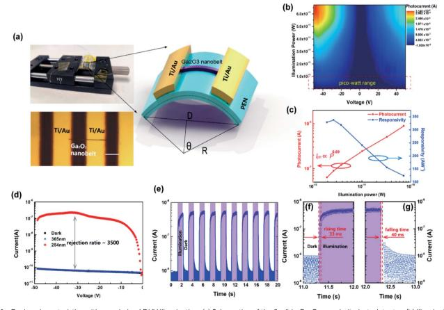
Fig. 2 Device characteristics with unpolarized DUV illumination. (a) Schematics of the flexible  $Ga_2O_3$  nanobelt photodetector. (b) Illumination – power-dependent I-V characteristics. (c) Diagram of photocurrent and responsivity versus illumination power. (d) Photocurrent under UV254 nm irradiation compared with that under UV365 nm irradiation. (e) Time-resolved photoresponse characteristics with V = 50 V. (f) Rising and (q) falling edge of one photoresponse cycle.
