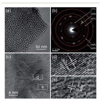
Fig. 3 (a) TEM image, (b) SAED pattern, (c) HRTEM image, and (d and e) magnified HRTEM images of the MgCo $_2$ O $_4$  NFs.
