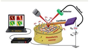
Scheme 2 Schematic representation of in situ SKPM imaging performed for  $ZnO@ln_2O_3$  heterojunction nanowires in the  $NO_2$  gas environment.
