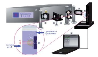
Fig. 1 The schematic of the laser ablation set up; 1: femtosecond laser system, 2: mirror, 3: polarizer, 4: beam splitter, 5 & 6: reflecting mirrors, 7: parabolic focusing mirror, 8: target position on motorized XYZscanning stage, 9: CNC controller program and 10: nanoparticle synthesis procedure (cavitation bubble expansion along with the formation of up-flow vapour bubbles).
