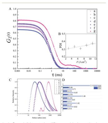
Fig. 9 Dynamic light scattering of Si nanoparticles in organic solvents; (A) autocorrelation function curves *versus* delay time; (B) PDI *versus* F for Si NPs in ethanol; (C) relative scattered intensities *versus* Stokes radius for Si NPs in various organic fluids; (D) comparison of PDI with IQR values; a, b, c, d and e: Si NPs in ethanol; f: Si NPs in 2-butanol; g: Si NPs in *n*-hexane.
