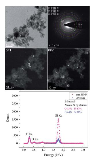
Fig. 6 The femtosecond laser-synthesized Si nanoparticles in 2-butanol. (N=1000, F=4.42 J cm $^{-2}$ ). The BF-TEM image (upper left), SAED pattern (upper right) and the DF-TEM images related to different diffracted electron beams along the  $1^{\rm st}$  and  $2^{\rm nd}$  ring. The EDX spectrum of several Si NPs shown in the BF-TEM and that of one single Si NP.
