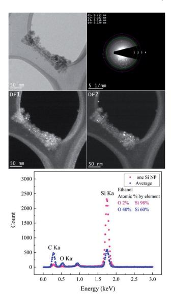
Fig. 4 The femtosecond laser-synthesized Si nanoparticles in ethanol.  $(N=1000, F=4.90~\mathrm{J~cm^{-2}})$ : BF-TEM image (upper left), SAED pattern (upper right) and DF-TEM images related to different diffracted electron beams along the 1<sup>st</sup> ring. The EDX spectrum contains an average of several Si NPs and one of a single Si NP.
