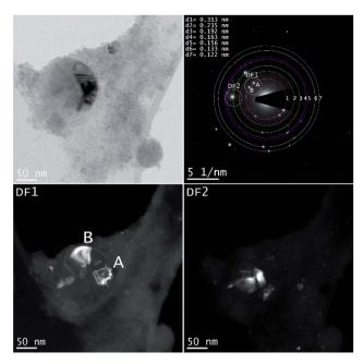
Fig. 5 The femtosecond laser-synthesized Si nanoparticles in ethanol. (N=1000,  $F=10.78~\rm J~cm^{-2}$ ). The BF-TEM image (upper left), SAED pattern (upper right) and the DF-TEM images related to different diffracted electron beams along the 1st and 3rd ring.
