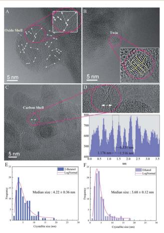
Fig. 8 HRTEM images of nanocrystalline Si NPs; (A) atomic orientations of an ultrafine-grained Si NP with an amorphous oxide shell in ethanol (N=1000, F=4.90 J cm $^{-2}$ ), (B) twin boundary defect in a Si NP in ethanol, (C) Si NP in 2-butanol (N=1000, F=4.42 J cm $^{-2}$ ) with a few atomic layers of the graphite shell, (D) zoom plot of graphite fringes with respective HRTEM profiles, (E) study of the average crystallite size of Si NPs in 2-butanol.
