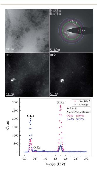
Fig. 7 The femtosecond laser-synthesized Si nanoparticles in nhexane. (N = 1000, F = 10.46 J cm<sup>-2</sup>). The TEM bright-field image, SAED pattern (upper right) and dark-field images related to different diffracted electron beams along the 1<sup>st</sup> and 2<sup>nd</sup> ring. The EDX spectrum from several small Si NPs and one Si NP.
