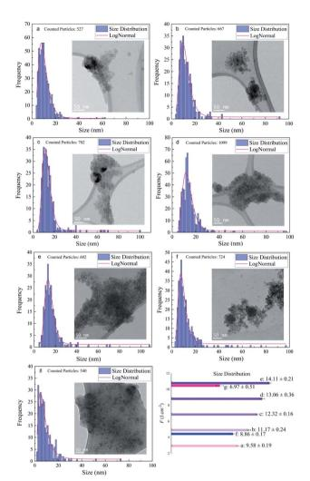
Fig. 3 Feret size distribution study of femtosecond laser synthesized silicon nanoparticles ( $N=1000, 1\,\mathrm{kHz}$ ); (a) ethanol,  $F=2.94\,\mathrm{J\,cm^{-2}}$ , (b) ethanol,  $F=4.90\,\mathrm{J\,cm^{-2}}$ , (c) ethanol,  $F=6.86\,\mathrm{J\,cm^{-2}}$ , (d) ethanol,  $F=8.82\,\mathrm{J\,cm^{-2}}$ , (e) ethanol,  $F=10.78\,\mathrm{J\,cm^{-2}}$ , (f) 2-butanol,  $F=4.42\,\mathrm{J\,cm^{-2}}$ , and (g) n-hexane,  $F=10.46\,\mathrm{J\,cm^{-2}}$ .
