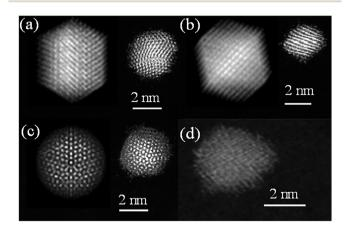
Fig. 3 Comparison between the simulated STEM images and the experimental ones for different structures. (a) On the top left corner is the simulated STEM image of a Dh structure, while the top right one is an experimental result. (b) The simulated STEM image and an experimental result of an Fcc structure. (c) The simulated STEM image and an experimental result of an Ih structure. (d) The experimental STEM images that cannot match with each simulated STEM ones.
