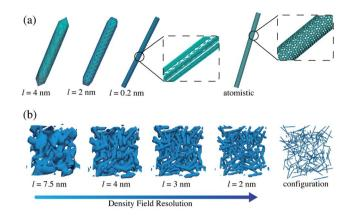
Fig. 3 Panel (a) single CNT isodensity surface at different grid sizes and CNT atomistic picture. Panel (b) isodensity surfaces of CNTs in random conformation at different grid sizes. A snapshot of CNTs in coarse-grained representation is also shown to quantify the different degree of detail reached at different grid sizes. In the figure, l represents the grid length.
