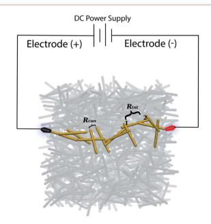
Fig. 1 Schematic picture of the CNTs forming a conductive path. A continuous network of CNTs is formed when the percolation threshold is reached. To measure the Joule heating power, the sample is placed between two electrodes and an external potential is applied. A thermocouple allows to evaluate the temperature increase. Both electrical resistances contributions to the percolative path, the intrinsic  $(R_{\rm int})$  and contact one  $(R_{\rm con})$ , are emphasized.
