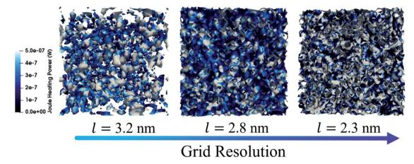
Heating power isosurface at different grid resolutions
