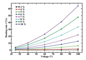
Fig. 9 Heating rate for the random CNT configurations at different applied voltages. The heating rate is shown for different CNT concentrations.
