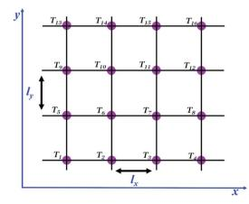
Fig. 7 Simplified schematic 2D picture of a  $4\times4$  grid to illustrate the grid scheme used to calculate local temperatures according to eqn (9) where the Joule heat contribution depending on the local CNT density is added. Temperatures are evaluated on the grid vertices. Periodic boundary conditions are applied in all directions. For this reason grid points 1 and 4, 5 and 8, 9 and 12, 13 and 16, 2 and 14, 3 and 15 are equivalent.
