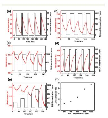
Fig. 5 Dynamic response-recovery curves of the gas sensor based on uranium dioxide nanoparticles towards (a) 20 ppm NO<sub>2</sub>; (b) 1000 ppm EtOH; (c) 1000 ppm CO; (d) 500 ppm NH<sub>3</sub>; and (e) varying CO concentration; (f) CO sensing response as a function of gas concentration. For measuring the NO<sub>2</sub> response, a 200 sccm N<sub>2</sub> flush was used for 1 h to recover the baseline.
