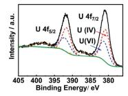
Fig. 6 High resolution U 4f XPS spectrum of uranium dioxide nanoparticles derived from the microwave decomposition of the uranyl EG gel. The spectrum was fitted with peaks of U(IV) and U(VI) (dashed lines).
