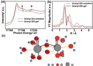
Fig. 2 (a) XANES (L<sub>3</sub>-edge of uranium) and (b) EXAFS spectra of uranyl EG solution and uranyl EG gel; FT peak positions are not corrected for phase shifts. A and B show features related to the axial and equatorial U-O bonds, respectively. (c) The scheme of the elongation of the U- $O_{ax}$  bond length and the shortening of the  $U-O_{eq}$  bond length of the hydroxo species in the gel phase.
