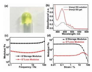
Fig. 1 (a) The photograph of the uranyl EG gel. (b) The UV-Vis absorption spectra of the uranyl EG gel and the uranyl EG solution. (c) and (d) The reheology properties of uranyl gel. (c) Dependence of the dynamic storage modulus (G') and loss modulus (G'') on the frequency at a constant strain of 0.5%. (d) Dependence of the dynamic storage modulus (G') and loss modulus (G'') on the strain at a constant frequency of 1 Hz.
