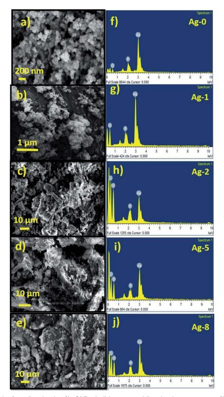
Fig. 2 FESEM micrographs of pure silver phosphate [Ag-0 (a)] and cellulose supported silver phosphate nanostructures [Ag-1 (b)], [Ag-2 (c)] [Ag-5 (d)] and [Ag-8 (e)] and their respective EDAX patterns (f-j).
