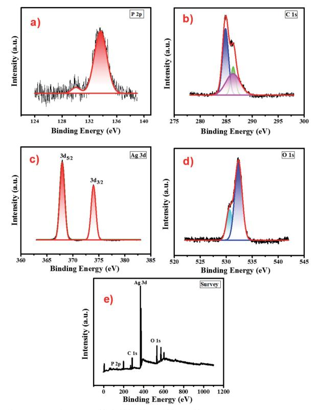
Fig. 4 XPS spectra of the Ag-8 photocatalyst (a) P 2p (b) C 1s (c) Ag 3d (d) O 1s and (e) survey scan.
