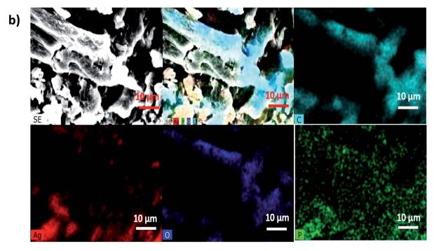
Fig. 1 (a) X-ray diffraction patterns of cellulose supported  $Ag_3PO_4$  nanostructures [Ag-0-Ag-8]. (b) SEM-EDX mapping images of cellulose supported silver phosphate nanostructures (Ag-8).
