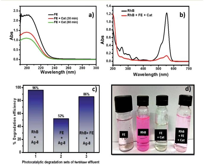
Fig. 7 (a) Photodegradation of fertilizer effluents using Ag-8 nanostructures. (b) Photodegradation of the fertilizer effluent and RhB dye with Ag-8 nanostructures. (c) Bar diagram of photocatalytic degradation of different sets. (d) Colour change before and after photodegradation.
