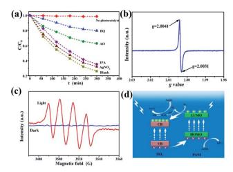
Fig. 7 (a) Kinetics of As(III) photocatalytic oxidation in the presence of different free radical trapping reagents. ESR spectra of the  $\gamma\text{-Fe}_2\text{-}O_3$ @PANI@TiO $_2$  for (b) light generated holes and (c) DMPO- $^{\bullet}O_2^{-}$ . (d) Schematic illustration of the postulated mechanism of As(III) photocatalytic oxidation on the  $\gamma\text{-Fe}_2O_3$ @PANI@TiO $_2$ .
