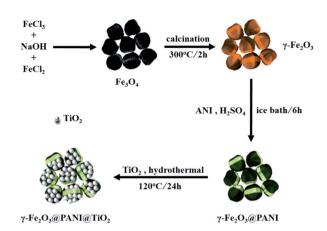
Fig. 1 Schematic illustration of the preparation procedure of  $\gamma\text{-}\text{Fe}_2\text{O}_3\text{@PANI@TiO}_2.$
