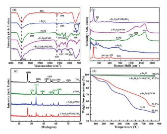
**Fig. 2** Characterization of TiO<sub>2</sub>,  $\gamma$ -Fe<sub>2</sub>O<sub>3</sub>,  $\gamma$ -Fe<sub>2</sub>O<sub>3</sub>@PANI, and  $\gamma$ -Fe<sub>2</sub>O<sub>3</sub>@PANI@TiO<sub>2</sub>: (a) FTIR spectra, (b) Raman spectra, (c) XRD spectra, and (d) thermogravimetric analysis (TG) curves.
