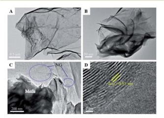
Fig. 8 TEM images of the samples (A–D): (A), N-doped graphene (NG); (B), MoS<sub>2</sub>; (C), MoS<sub>2</sub>/NG; (D) high-resolution image of MoS<sub>2</sub>/NG. Reprinted from ref. 47. Copyright 2020, with permission from Elsevier.
