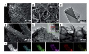
Fig. 11 (A) Low, (B) high-resolution FESEM, and (C) TEM image of TiO<sub>2</sub> CNBs. (D) FESEM, (E) TEM, and, (F) HRTEM images of MoS<sub>2</sub>@TiO<sub>2</sub> CNBs. (G) EDS elemental maps of Ti, O, Mo, S, and C, respectively. Reprinted from ref. 46. Copyright 2017, with permission from Elsevier.
