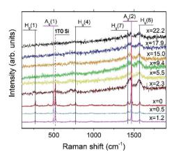
Fig. 9 Raman spectra of the  $Au_xC_{60}$  films with different Au concentrations (x). The x values are shown for the respective spectra. Some of the  $C_{60}$  vibration modes with  $A_g$  and  $H_g$  symmetry are indicated by vertical lines. The position of the intense 1TO Si(100) mode is indicated by the dashed vertical line (see text).
