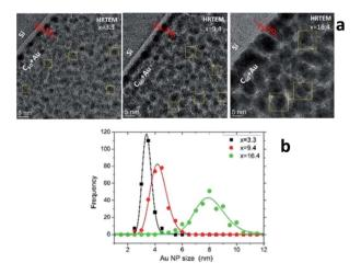
Fig. 4 (a) HRTEM images of samples S2, S5 and S8. The whitish strip between the Si substrate and Au<sub>x</sub>C<sub>60</sub> mixture film corresponds to native SiO<sub>2</sub> layer (about 2 nm in thickness). (b) Log-normal size distribution of the Au NPs in samples S2, S5 and S8 as obtained from the analysis of approximately 250 NPs per sample.
