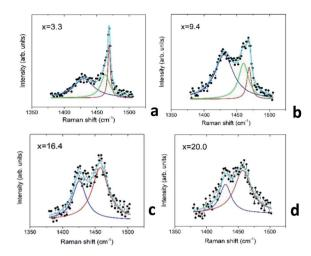
Fig. 10 Raman spectra of the  ${\rm Au_x C_{60}}$  mixture films near the positions of the  ${\rm H_g(7)}$  and  ${\rm A_g(2)}$  modes of  ${\rm C_{60}}$ : (a and b) the mixture films from the interval R2; (c and d) the mixture films from the interval R3. The experimental spectra (black dots) fitted by a superposition of Lorentzians (light-blue line). See description in the text.
