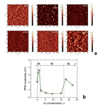
Fig. 2 (a) AFM images of the surface morphology of selected  $Au_xC_{60}$ films. The Au concentrations x in the films were added to the respective images. (b) Variation of the RMS surface roughness of the  $Au_xC_{60}$  films with increasing x. R1, R2 and R3 indicate three different x intervals in which the Au<sub>x</sub>C<sub>60</sub> nanostructures possess a common structural feature. Vertical dashed lines indicate the border (critical points,  $x_c$ ) between the intervals (see text)
