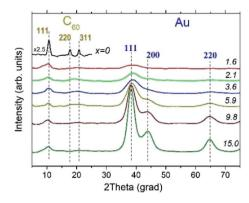
Fig. 6 XRD patterns of pure  $C_{60}$  film (x=0) and of  $Au_xC_{60}$  mixture films with different Au contents (x). The x values are shown in the plots. Experimental XRD patterns were smoothed prior to plotting, and the rapidly increasing background at smaller angles was subtracted.
