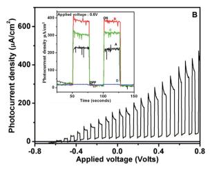
Fig. 4 Photocurrent–voltage curve of the film-B SRZO photoanode with chopped light illumination under a solar simulator (AM1.5G). The inset shows the comparison of the current transient with time for different SRZO photoanodes under on/off illumination.
