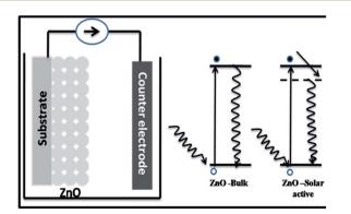
Fig. 7 Schematic showing the red-shift in the band gap of the SRZO photoanode compared to bulk ZnO.
