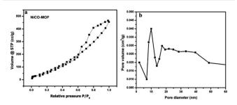
Fig. 5 (a) N<sub>2</sub> adsorption-desorption isotherms of the NiCo-MOF nanosheet array, and (b) the corresponding pore size determination of the NiCo-MOF nanosheet array.
