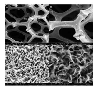
Fig. 2 FE-SEM images of NiCo-MOF/NF at various scales: (a) 500  $\mu$ m, (b) 300  $\mu$ m, (c) 10  $\mu$ m, and (d) 5  $\mu$ m.
