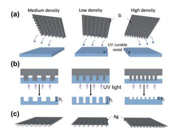
Fig. 2 Schematics of the UV-assisted nanoimprint lithography (UV-NIL) process: (a) a master mould consist of multiple density of nanoprotrusions used in the UV-NIL which results in the nanocavity with various imprinting depth,  $h_{\rm i}$  as depicted in (b). (c) Scheme showing the geometry of the Ag 'floating' resonance particle and metal back layer upon metal coating process. Height of the structures in the schematics are not to be scaled.
