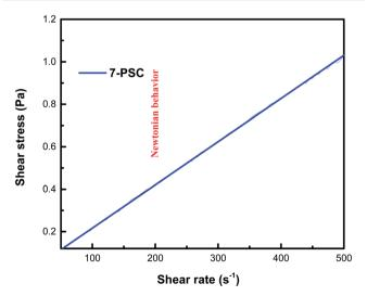
Fig. 13 Newtonian behavior of the 7-PSC/engine oil nanofluid.
