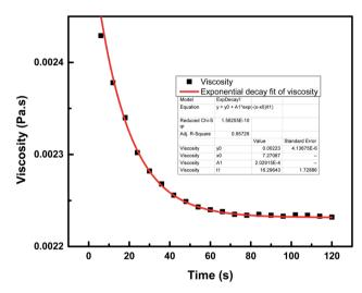
Fig. 10 Viscosity variation of 7-PSC in 15W-40 engine oil (base fluid) with time at a constant shear rate of 100 s<sup>-1</sup>.
