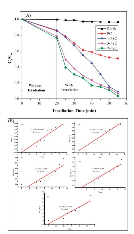
Fig. 6 (A) Percentage photodegradation of PBS dye in aqueous solution over the blank, PC, 1-PSC, 5-PSC, and 7-PSC nanocomposites in the presence and absence of visible light illumination. (B) The rate constants of the curve of the different photocatalysts against PBS dye: (a) blank test, (b) PC, (c) 1-PSC, (d) 5-PSC, and (e) 7-PSC.
