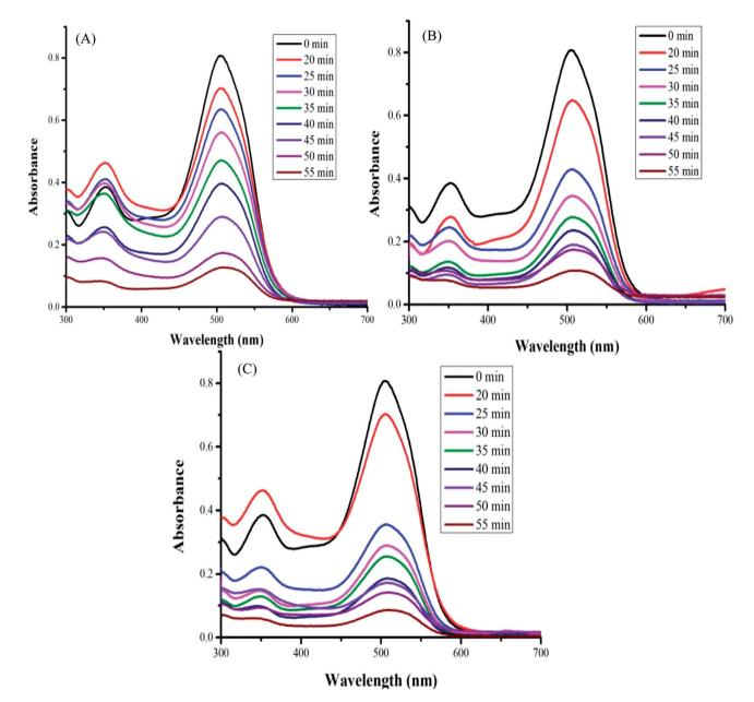
UV visible spectra of the samples of PBS dye degraded by the polymer nanocomposites (A) 1-PSC, (B) 5-PSC, and (C) 7-PSC
