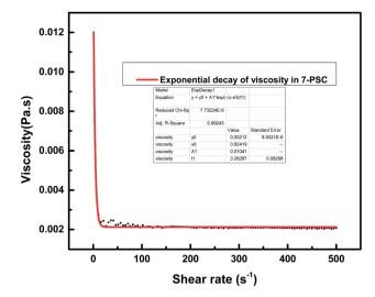
Fig. 12 Effect of shear rate on the viscosity of the 7-PSC nanocomposite dispersed in 15W-40 engine oil.
