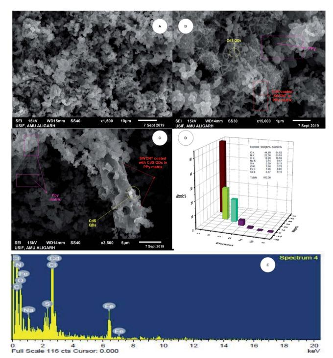
Fig. 2 SEM micrographs of (A) 1-PSC, (B) 5-PSC, and (C) 7-PSC. (D and E) EDX analysis.
