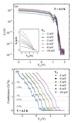
Fig. 8 (a) Transfer characteristics on the logarithmic scale of the devices fabricated from the Ge-core/a-Si shell nanowire with a channel length of 500 nm at low  $V_{\rm d}$  (-2, -4, -5, -6, -8 and -10 mV) at T=4.2 K. Inset: transfer characteristics on the linear scale. (b) Extracted conductances from (a) showing stepwise features at several  $G_0$  values including the quantization at  $\sim$ 0.7 $G_0$  ("0.7 structure"). The x-axis has been shifted to the right for clarity of comparison.
