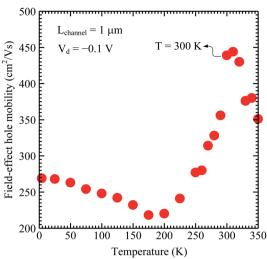
Fig. 7 Field-effect hole mobility *versus* temperature calculated at  $V_{\rm d}=-0.1$  V. The field-effect hole mobility value was selected at  $V_{\rm g}$  0.88 V for each temperature condition.
