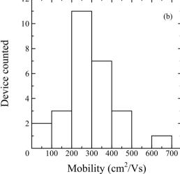
Fig. 4 (a) Field-effect hole mobility versus gate voltage  $(V_a)$  at  $V_d =$ -0.01, -0.1, -0.5 and -1 V. (b) Histogram of Ge-core/a-Si shell nanowire FET mobility.
