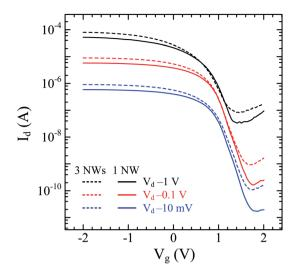
Fig. 5 Transfer characteristics ( $I_d$  versus  $V_g$  curve) of the devices consisting of a single nanowire (solid curves) and three nanowires (dashed curves) at a  $V_d$  of -0.01 V, -0.1 V and -1 V. The gate voltage  $(V_0)$  was swept from -2 to 2 V. The channel length is 1  $\mu$ m.
