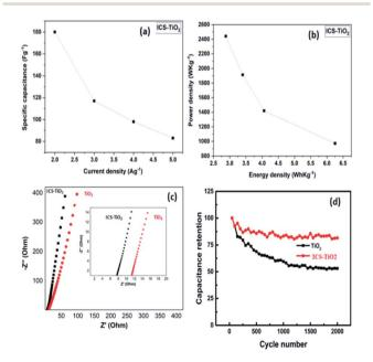
Fig. 6 (a) Specific capacitance vs. current density, and (b) power density vs. energy density for ICS-TiO2. (c) EIS spectra of TiO2 and ICS-TiO<sub>2</sub>; (d) cyclic stability of TiO<sub>2</sub> and ICS-TiO<sub>2</sub>.
