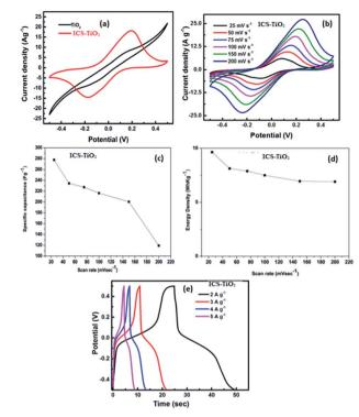
Fig. 5 (a) CV curves of  $TiO_2$  and  $ICS-TiO_2$  recorded at 100 mV s<sup>-1</sup>. (b) CV curves of ICS-TiO<sub>2</sub> recorded at scan rates of 25, 50, 75, 100, 150 and 200 mV s<sup>-1</sup>. (c) Specific capacitance as a function of scan rate; (d) energy density as a function of the scan rate of ICS-TiO<sub>2</sub>. (e) Charge and discharge curves of ICS-TiO<sub>2</sub> measured at current densities of 2, 3, 4, and 5 A  $g^{-1}$
