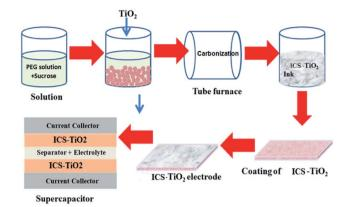
Fig. 1 Schematic of ICS-TiO<sub>2</sub>-based supercapacitors.
