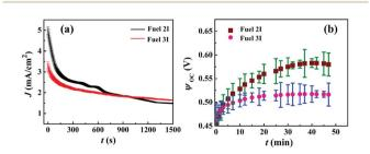
Fig. 4 (a) Chronoamperometric current density (*J*) versus time (*t*) studies for different  $\mu$ -DropFCs with the Fuels 2I and 3I at an applied voltage of 0.1 V. (b) The corresponding open-circuit potential ( $\psi_{oc}$ ) with *t* for 50 min. To demonstrate long-term performance of  $\mu$ -DropFCs, the chronoamperometry test was performed for different systems.
