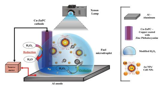
Fig. 1 Schematic of the  $\mu$ -DropFC setup comprising of a Cu–ZnPC cathode, an Al foil anode, a microdroplet with the fuel (0.3 M  $H_2O_2$ , 0.1 M HCl, 1 M NaCl), additives (Au/CdS NPs) and light source. The image also schematically shows the redox half-reactions at the cathode and anode,  $H_2O_2 \rightarrow O_2 + 2H^+ + 2e^-$  and  $H_2O_2 + 2H^+ + 2e^- \rightarrow 2H_2O$ , respectively. The legends aid in the identification of the different components and their placements.
