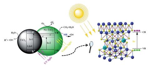
Fig. 7 Possible mechanism of the MB degradation by Ni-TiO<sub>2</sub> nanoparticles.
