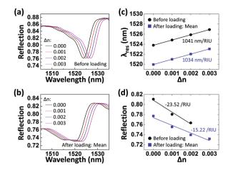
Fig. 8 Simulated reflection spectra of the on-fiber Au nanopatch array (a) before and (b) after thermal loading with respect to the changes in the refractive index of the optical fiber. (c) Simulated  $\lambda_{\rm res}$  shifts as a function of the refractive index change. (d) Simulated reflections at the 1526.31 nm and 1523.76 nm of wavelengths for the Au nanopatch array before and after thermal loading, respectively, as a function of the refractive index change.
