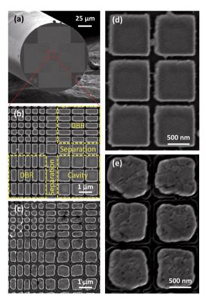
Fig. 6 SEM images of the fabricated Au nanopatch array on a singlemode optical fiber: (a) the fiber end-face with a plasmonic crystal cavity, a corner section of the plasmonic cavity (b) before thermal loading and (c) after 500 cycles of thermal loading, and the square Au nanopatches in the plasmonic cavity (d) before thermal loading and (e) after 500 cycles of thermal loading
