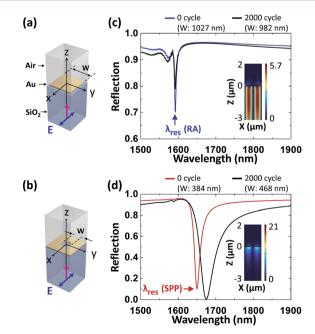
Fig. 5 Schematic of 3D unit cell simulation models for (a) square Au nanopatch array and (b) circular Au nanohole array (P = 1100 nm). Simulated reflection spectra of (c) the square Au nanopatch array and (d) circular Au nanohole array before thermal loading and after 2000 cycles of thermal loading. The insets show the electric field distributions ( $|E_z|$  at y=0) at the  $\lambda_{res}$  before thermal loading
