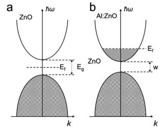
Fig. 2 The illustration of band structures of (a) ZnO and (b) Al:ZnO.
