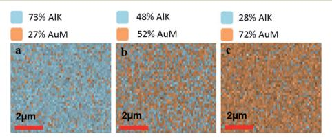
Fig. 1 (a-c) Energy dispersive spectroscopy (EDS) images representing the ratio of AlK/AuM emission from the surface of mixed metal ZMWs i.e. 75Al, 50Al and 25Al respectively. The ratio of Alk/AuM on the ZMW surfaces matches the target ratio of Al and Au in respective mixed metal ZMWs.
