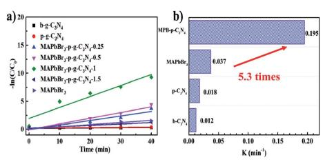
Fig. 6 (a) Photocatalytic kinetic behavior for the corresponding dependence of  $\ln(C/C_0)$  on irradiation time. (b) Comparison of slope values of different samples
