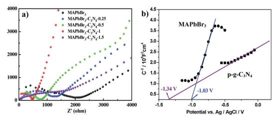
Fig. 9 (a) Electrochemical impedance spectroscopy (EIS) spectra of the MAPbBr<sub>3</sub>/p-g- $C_3N_4$  composites and (b) Mott–Schottky plot on MAPbBr<sub>3</sub> and p-g- $C_3N_4$ , showing n-type semiconducting features and flat band potentials of -1.03 V and -1.34 V vs. Ag/AgCl, respectively.
