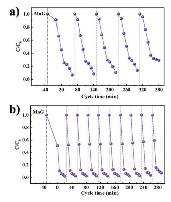
Fig. 11 (a and b) Long-term cycling stability tests of the MAPbBr<sub>3</sub> and MAPbBr<sub>3</sub>/p-g-C<sub>3</sub>N<sub>4</sub>-1.0 under visible-light irradiation for photoreduction of malachite green.
