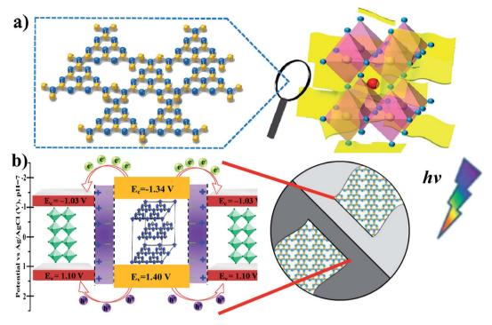
Fig. 10 (a) Schematic illustrations of the MAPbBr $_3$ /p-q-C $_3$ N $_4$  intergrowth microcrystal composite wrapped/entrapped nanosheets on the molecular level. (b) The proposed corresponding inverted type-I band configuration structure alignments of MAPbBr<sub>3</sub> and p-g-C<sub>3</sub>N<sub>4</sub>, which are similar to core/shell heterostructure band structures.
