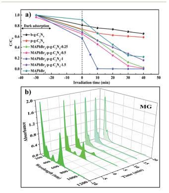
Fig. 5 (a) Photocatalytic activities of concentration—time profiles of the degradation of MG over various catalysts including b-g-C<sub>3</sub>N<sub>4</sub>, p-g-C<sub>3</sub>N<sub>4</sub>, MAPbBr<sub>3</sub>, and MAPbBr<sub>3</sub>/p-g-C<sub>3</sub>N<sub>4</sub> samples under visible light. (b) 3D UV-vis spectra of malachite green (MG) at different irradiation times in the presence of the MAPbBr<sub>3</sub>-p-g-C<sub>3</sub>N<sub>4</sub>-1.0 mg sample.
