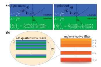
Fig. 1 (a) Diagram of p-polarized and s-polarized light at the interface of two media. (b) Geometry of a broadband angle selective filter based on N quarter-wave stacks of increasing thickness. Each quarter-wave stack is conformed by M bilayers satisfying the Bragg condition.
