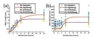
Fig. 4  $\,$  ZnO NWs' (a) length and (b) diameter as a function of growth time; the growth temperature has been fixed at 90  $\,$  °C and the precursor's concentration has been fixed at 40 mM.
