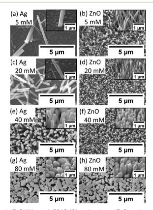
Fig. 7 ZnO NW growth (90 °C, 18 hours) on Ag and ZnO seed layers as a function of different precursor concentrations (top view and tilted 45°). On the Ag seed layer: (a) 5 mM, (c) 20 mM, (e) 40 mM, and (g) 80 mM; on the ZnO seed layer: ZnO (b) 5 mM, (d) 20 mM, (f) 40 mM, and (h) 80 mM.
