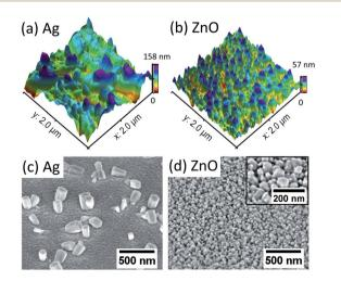
Fig. 1 AFM and SEM (top view) images of the initial state (40 mM, 90 °C, 0.5 hours) ZnO nanocrystals grown on the 50 nm patterned Ag seed layer (a) and (c); ZnO seed layer (b) and (d). In (d), the high magnification SEM image is shown in the inset
