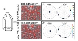
Fig. 2 EBSD result of ZnO NWs grown on Ag and ZnO seed layers at 40 mM, 18 hours, and 90 °C. (a) Idealized growth habit of the ZnO crystal (adapted from ref. 39: W. J. Li et al., J Cryst Growth, 1999). Electron diffraction pattern of a single point detected on ZnO NWs: (b) ZnO NWs grown on Ag and (d) ZnO NWs grown on ZnO. Pole figures of the (0001) crystal facet and (1010) crystal facet, mapped from a single ZnO grain: (c) ZnO NWs grown on Ag and (e) ZnO NWs grown on ZnO.
