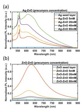
Fig. 10 PL spectra of ZnO NWs grown on (a) Ag and (b) ZnO seed layers as a function of precursor concentration (growth time of 18 hours)
