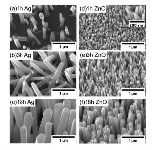
Fig. 5 ZnO NWs grown as a function of different times ( $45^{\circ}$  tilted, temperature of 90 °C, precursor concentration of 40 mM), on Ag: (a) 1 hour, (b) 3 hours, and (c) 18 hours; on ZnO: (d) 1 hour with the high magnification image in the inset, (e) 3 hours, and (f) 18 hours.
